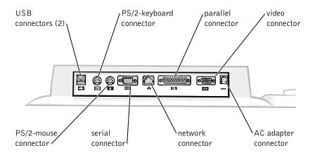
The "External I/O Connectors" table shows the icons for each of the connectors on the back of the APR and indicates the type of external device(s) that you can attach to each connector.
