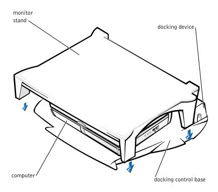
**NOTE:** Be sure that the back legs on the monitor stand engage the slots on either side of the docking control base.
